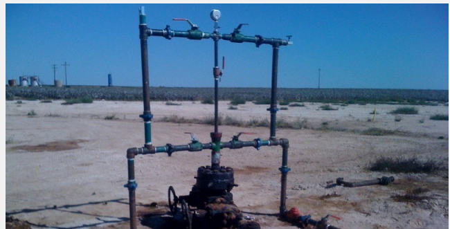
1" x 2.375" Slimhole Jet Pump Well Head
